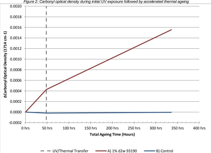
Figure 2: Carbonyl optical density during initial UV exposure followed by accelerated thermal ageing
